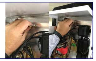
NB. Anodes can only be effective when fitted correctly and used where corrosion from galvanic reactions exist. Anodes can only assist in reducing corrosion, other factors may require additional protection or consideration.
